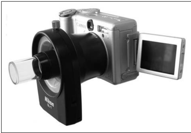
Figure 2. Canon Powershot A95 equipped with optics for skin contact microscopy.
