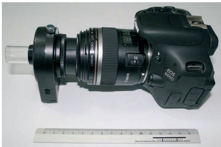
**Figure 10.** Canon EOS 600 camera with Canon macro and adjusted TrichoScan-optics for highest resolution images from the scalp.
