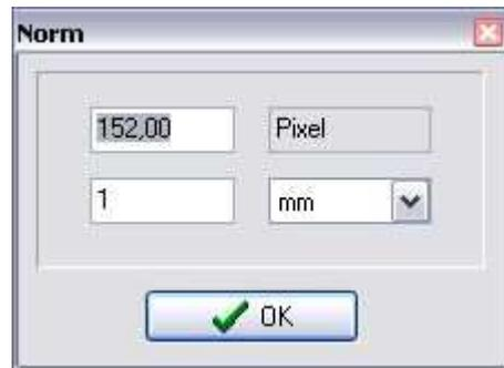
**If the image scale for a recording system is known it can be entered directly into the scale window as a number in unit pixels/mm.**
